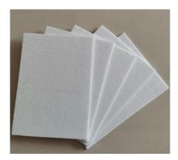
Aerogel Composite Insulation Board is a board made of aerogel and polystyrene. The results show that the addition of aerogel is 1.6-2.0%, and the thermal conductivity is reduced from 0.043w/m.k of pure polystyrene board to 0.0248w/m.k, improving the thermal insulation effect and flame retardancy.
